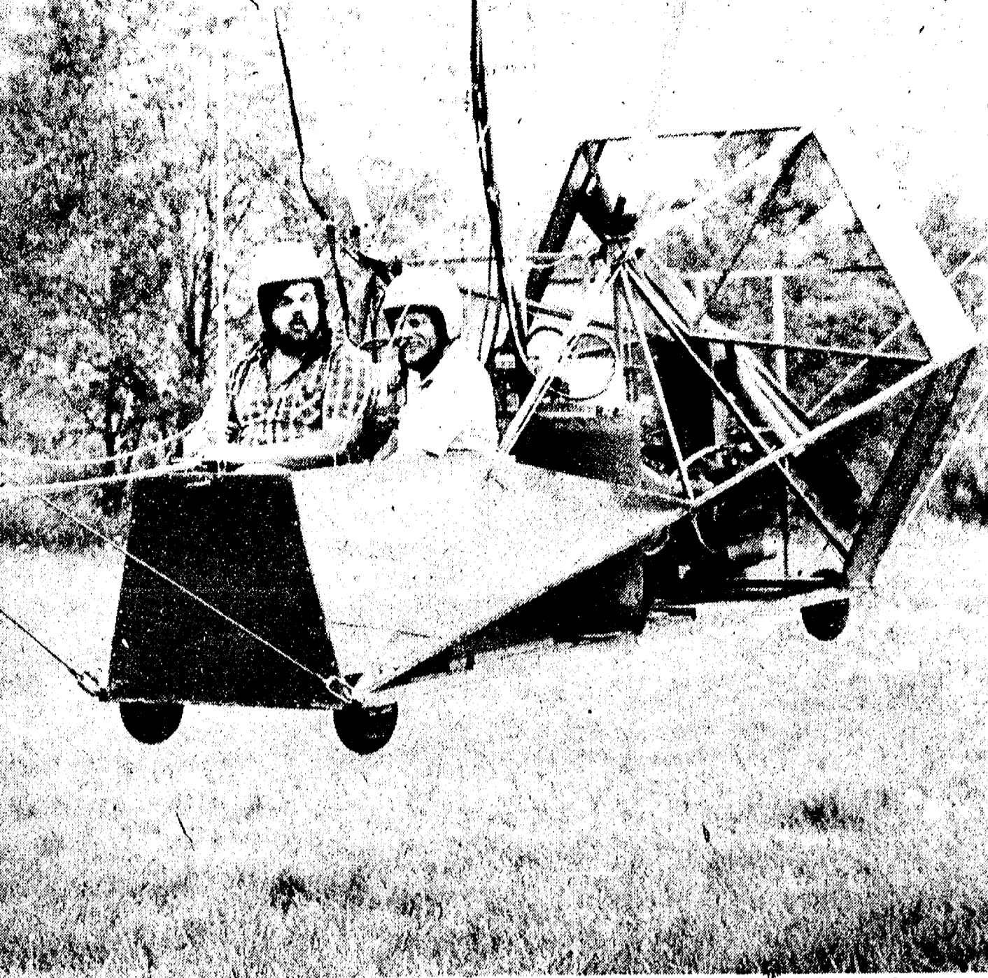
UP, UP AND AWAY: All by itself, this tiny car looks like an experimental model of a new kind of airplane. Attached to all the lines and cables, however, is a huge envelope containing 140,000 cubic feet of hot air. A Volkswagen engine turns the 5 1/2 foot propeller in the rear, which maneuvers the craft and provides a little bit of lift. Pilot and passenger are half of the Swedish team that brought the airship to Chelsea early this week.
