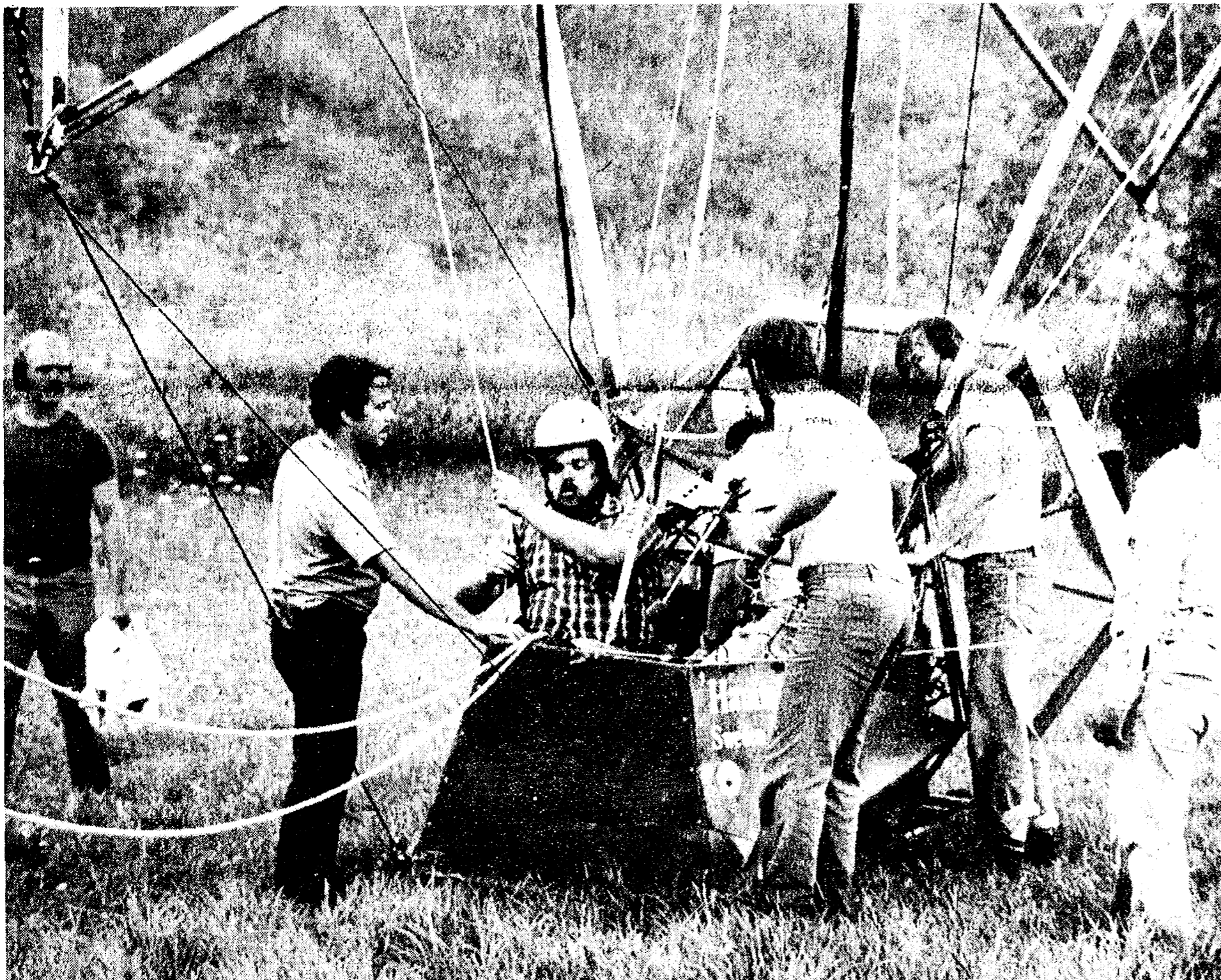
PRE-FLIGHT CHECK: Two visitors from Sweden prepare to ascend in this uncommon, blimp-shaped hot air balloon that startled a number of local residents as it flew near the Chrysler Proving Grounds early Monday. The complex network of metal rods and cables attaches this small gondola to an envelope 130 feet long and 65 feet high. A number of local balloon enthusiasts took rides in the small gondola — one at a time.
